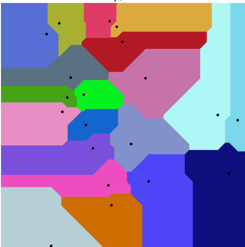
Zone map that was constructed for 20 hospitals (the locations of which were indicated with a black dot), with distances calculated based on the Manhattan distance.
